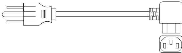
**Cable #2: For Printer Operation PC (125VAC, 15A, 10.2 ft with straight inlet plug).**
