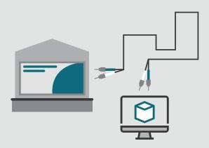
Each fiber configuration uses an indoor controller and requires that the cable be run through a 1.5" conduit to the sign. Closed-loop systems can be customized to meet security needs and PC-based software is required. Select interior displays in sports and event venues may use Cat 5/6 cable for communication.
